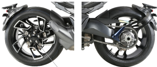
M12×1.5 nuts Rear wheel nut tightening torque: 110N.m
